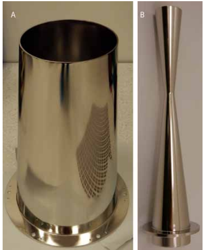
Figure 11 (a) Cone between DPA chambers 1 and 2; (b) Cone between DPA chambers 2 and 3.
