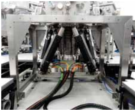
Figure 7 Hexapod and bellow installed underneath the exposure chamber.
