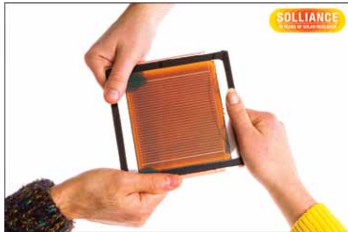
Figure 3 Glass/glass encapsulated perovskite module with an aperture area of 100\text{cm}^2 and efficiency above 10%, developed by Solliance Solar Research and collaborators [15]. The module withstands 1000 hrs continuous illumination at 1 Sun, 1000 hrs exposure to high humidity and 50 thermal cycles from -40 to 85^\circ\text{C} . The thermal ALD \text{SnO}_2 (TU/e) plays a major role in protecting the perovskite absorber during the thermal test. Acknowledgement for the photograph: Niels van Loon (Solliance Solar Research).
